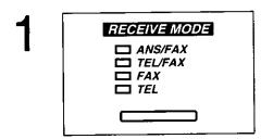
Press the **RECEIVE MODE** button until the ANS/FAX indicator lights.
