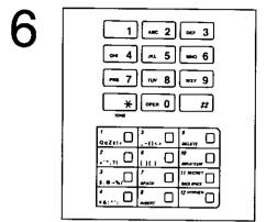
Enter the name associated with the speed dial station by using the dial keypad and the direct call station keys as character keys, and the cursor keys.
