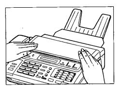
Close the paper compartment cover carefully by pressing down on both ends gently.
