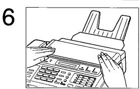
Close the recording paper unit carefully by pushing down on both ends gently.
