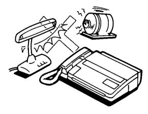
The unit and the cassette tape should be kept free from dust, moisture, high temperature and vibration.
