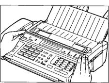
Then close the document feeder unit carefully by pushing down on both ends gently.
