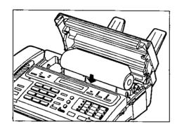
Place a recording paper roll into the paper compartment.
