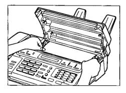
Pull the paper a few centimeters (one or two inches) out of the unit.
